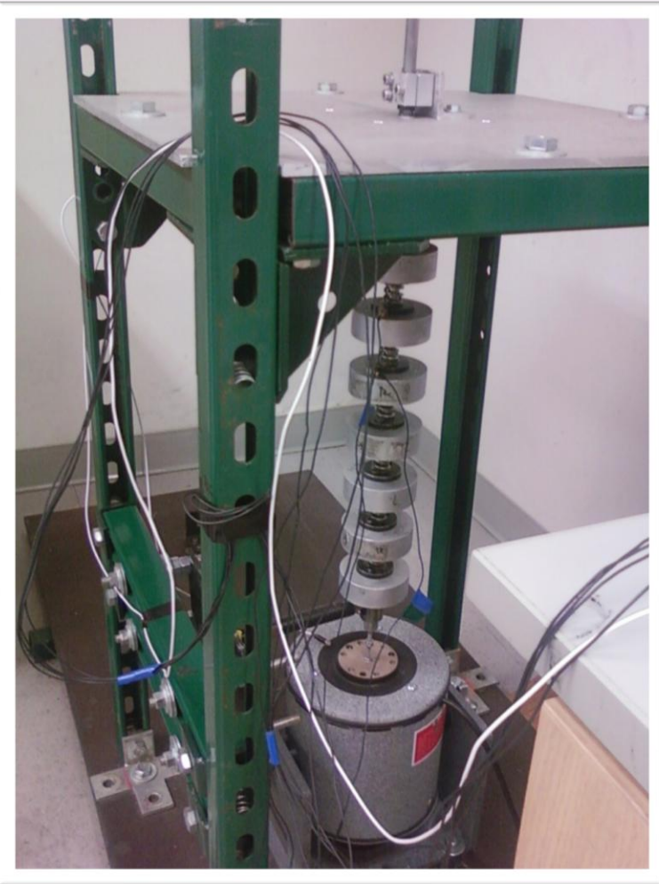
Using hyperchaotic interrogation for damage detection of an 8DoF system
